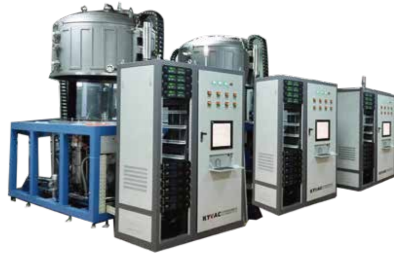
多工位真空镀膜及封接检测设备 Multi station vacuum coating and sealing detection equipment
