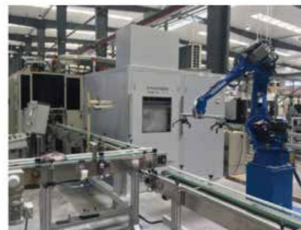
真空氦检漏设备 Vacuum helium leak detection equipment
