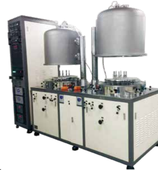
激光陀螺充排气设备 Charging And Discharging Device Of Laser Gyro
